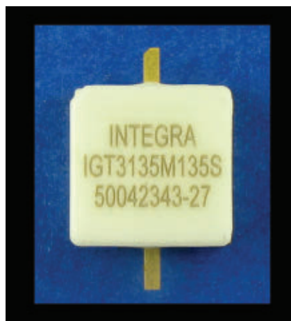
▲ Fig. 2 S-Band (3.1 to 3.5 GHz) 135 W GaN transistor internally matched to 50 \Omega . Package size is 0.4" \times 0.4".
