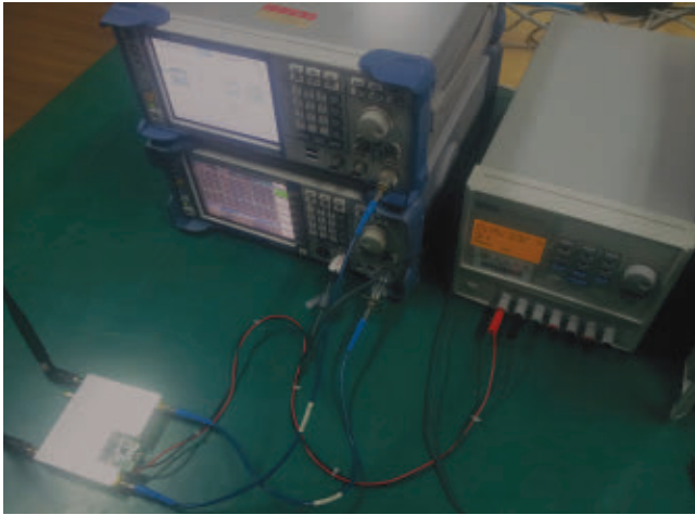
▲ Fig. 6 Setup for measuring RF self-interference cancellation performance.
