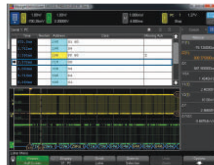
▲ Fig. 3 Serial communications can be decoded and analyzed with protocol analysis tools.
