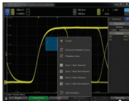
▲ Fig. 2 Zone triggering enables isolating a signal with a non-monotonic edge.
